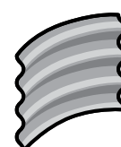
Each circle of galvanised iron is composed of three curved sections bolted together
